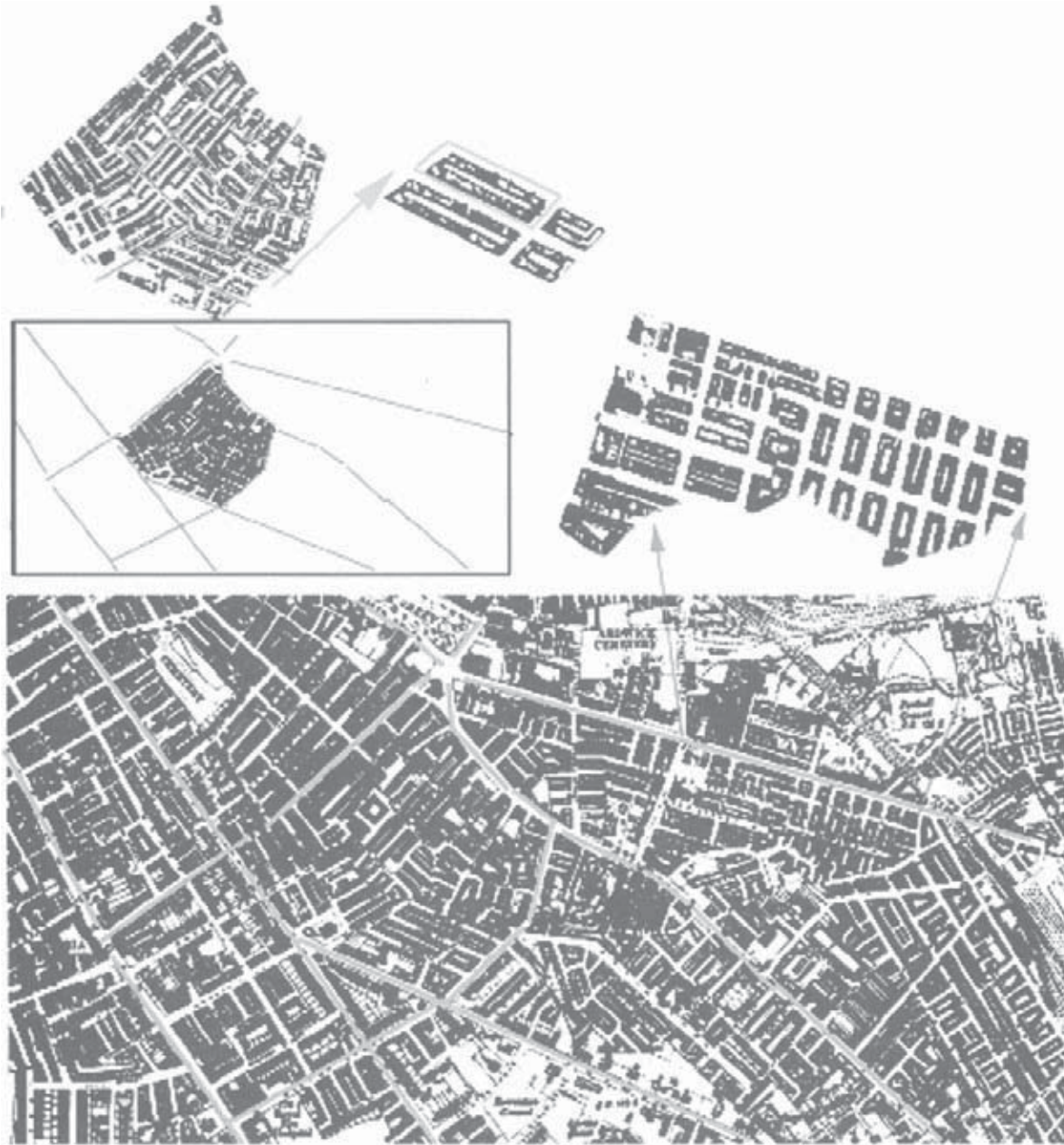
Fig. 9. Manchester, England. The urban patterns in Manchester do not offer such an abundance of features as Milan's (Fig. 8). Major and secondary roads create districts with common structural elements. The resulting definition of the internal blocks of the district can be simply understood. The block is defined by repetition, size and geometrical direction, and by regularity of plot dimensions.
